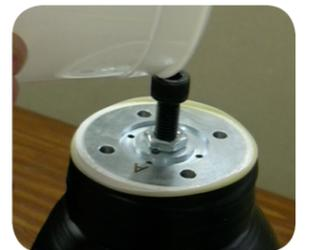
17. To create the Distal Pad, pour the resin into the hole in the screw until the resin is visible through the 4 vent holes. Let cure for 30-45 minutes.
