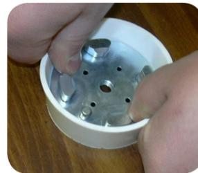
6. Heat the Sleeve with a heat gun until the Sleeve becomes pliable. Lift the Sleeve off of the Base.
