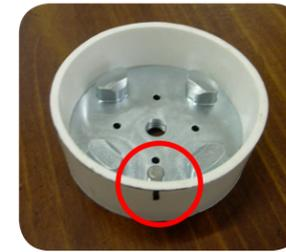
10. Spray the Sleeve/Base assembly with a urethane mold release or coat with petroleum jelly. Do not use a silicone mold release.
