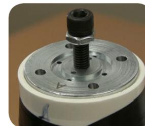
15. Spray urethane mold release onto the surface of the Tooling Base.
