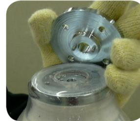
27. Remove the plastic to expose the head of the 1/4 x 20 screw.
