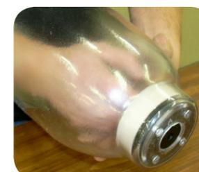
38. Using the four M6 x 55 screws provided, install the LimbLogic Vacuum Pump with the two Proximal Gaskets between the pump and the Drop-In Adapter and with the on/off button oriented correctly. Tighten the screws to 9 ft-lbs (12 Nm).
