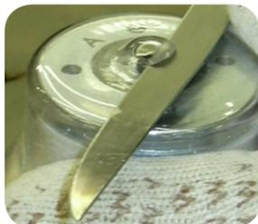
33. Insert the 10 mm cap screw into the Tooling Cap and Base. Use the hex nut to tighten the cap. It may be necessary to use a heat gun or torch to re-heat the Forming Cap. Allow to cool.
