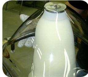
32. **Wearing heat-protective gloves,** remove the heated Cap from the oven and place it on the model. Align the two pins in the Cap with the holes in the Base.
