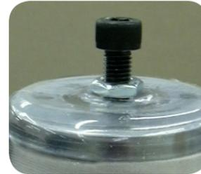
24. Apply Nysert and tie off around the 1/4" cap screw. Reflect the rest of the Nysert back onto the model.
