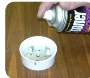
11. Stretch the Latex Form onto model, secure it, and spray it with mold release.
