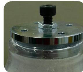
34. Using the Forming Cap as a drill guide, drill the 4-hole pattern. Remove the cap screw and the Forming Cap.
