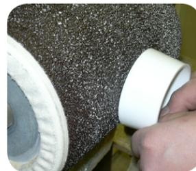
5. Press the Base into the sanded Sleeve.
