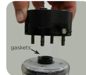
**Note: Due to the possibility of compression set of the thermoplastic, check the torque of the four M6 x 55 screws after two weeks of use.**
